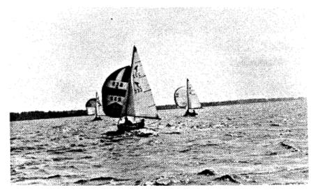
The spinnaker is your most versatile sail. It develops aerodynamic forces in varying degrees in all situations. The angle of attack at the luff is vitally important to ensure forces are generated in the optimum direction. The shape of the sail is also critical depending on your course off the wind. Ideally, the spinnaker should be full for dead downwind work and relatively flat for a close reach. This poses a problem because for this reason you would ideally want two spinnakers. To prevent
